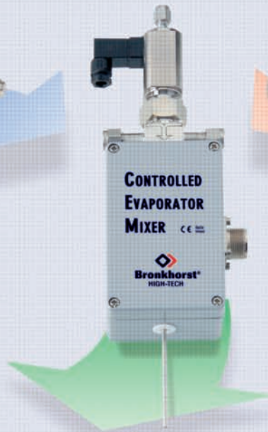
CEM Mixing chamber for liquid and carrier gas with heat exchanger for total evaporation
