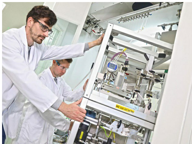
Bronkhorst Liquid Dosing skid (copyright: ISPE)
