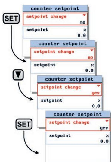
When entering the counter setpoint settings screen the setpoint change parameter is selected. Press **SET** to enter the edit mode.
