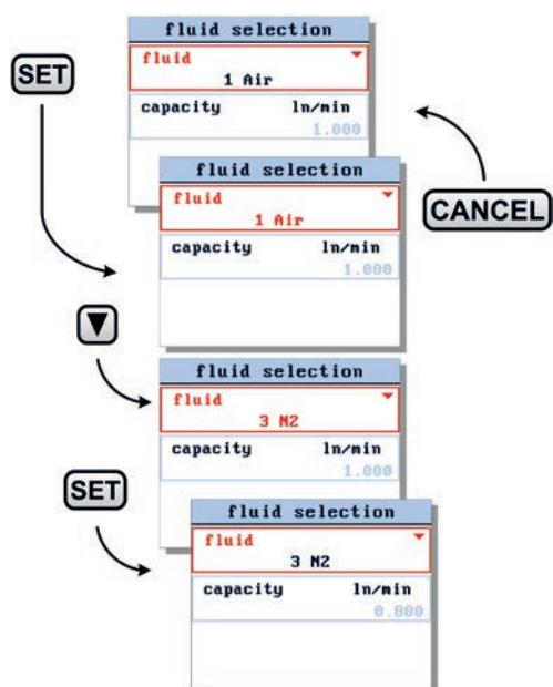
Press **SET** again to enter the edit mode of the fluid field. Use **▲** or **▼** to select one of the available fluidsets. Press **SET** to confirm.
