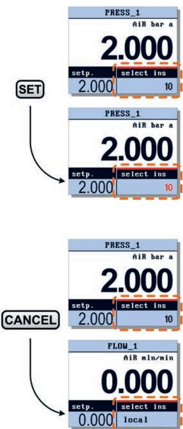
Press **SET** to select this instrument to be operated by the BRIGHT or press **CANCEL** to return to the previous selected instrument.
