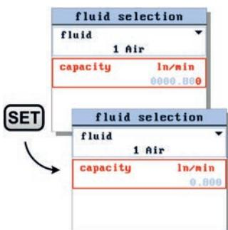
Now the fluid capacity can be changed between the minimal and maximal capacity of the selected fluid of the operating instrument.
