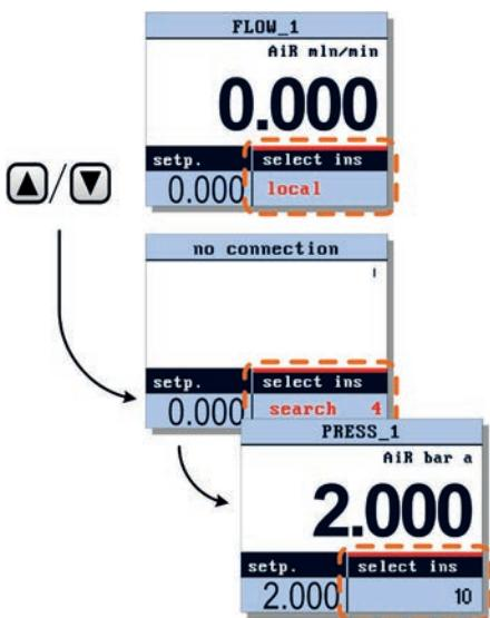
The instrument directly connected with the BRIGHT will be indicated as 'local'. Other instruments will be indicated with their node address.
