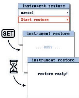
Press **SET** to start the instrument restore procedure. While the restore procedure is active, the BRIGHT will show the message 'busy'. When finished, 'auto restore ready'. Press any key to return to settings menu.
