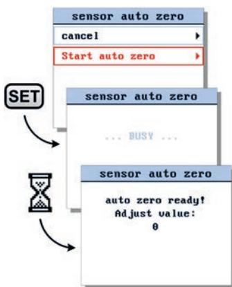
Press **SET** to start the sensor auto zero procedure. While the auto zero procedure is active, the BRIGHT will show the message 'busy'. When finished, 'auto zero ready'. Press any key to return to settings menu.
