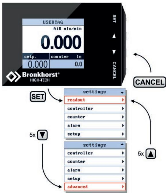
From the readout screen press **SET** to enter the settings menu. Press **CANCEL** to return to the readout screen.
