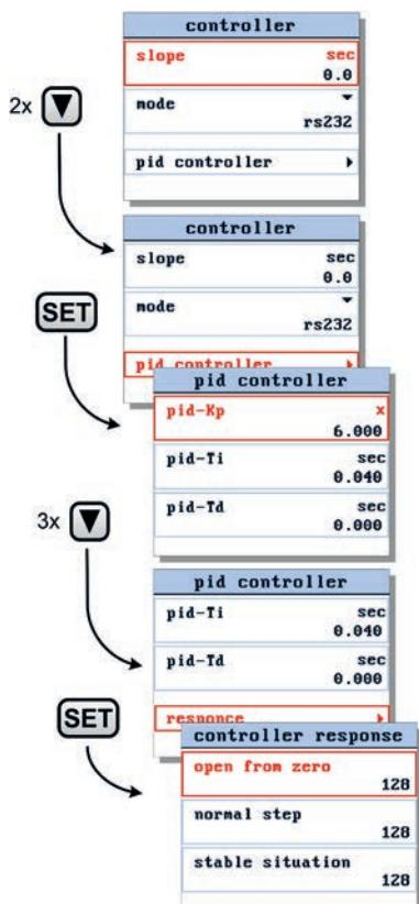
To edit these parameters, select the the 'pid controller' and press **SET**. In the pid controller settings screen select the option response and press **SET** to enter.
