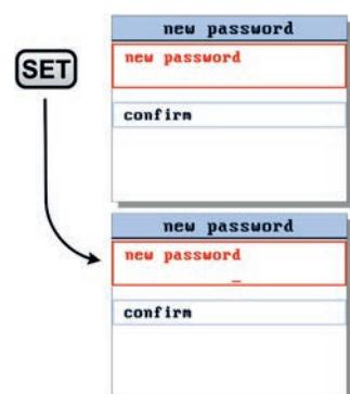
This will open the 'new password' input display. Press **SET** again to enter the new password edit mode.
