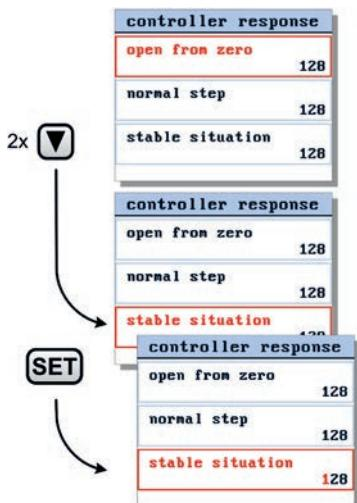
In the controller response settings screen you can select one of the parameters using the **▲** and **▼** buttons. Press **SET** to enter the edit mode.
