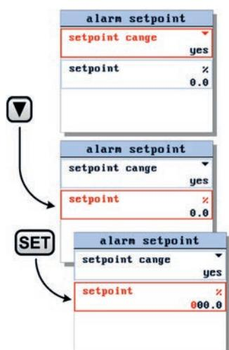
In the alarm setpoint settings screen press **▼** to select the setpoint parameter. Press **SET** to enter the edit mode.
