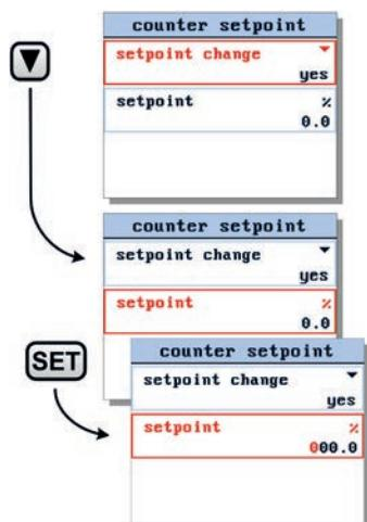
In the counter setpoint settings screen press ▼ to select the setpoint parameter. Press **SET** to enter the edit mode.
