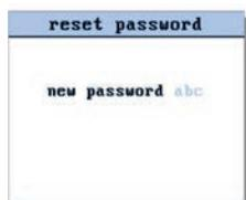
Again press both **▲** and **▼** for 5 seconds till the 'reset password' display appears.
