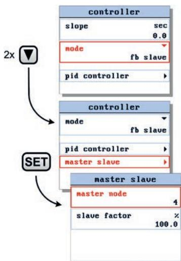
To enter the master slave settings screen, select the master slave option from the controller settings screen and press **SET** to enter.
