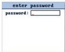
The default password is 'abc'. The password can consist of a maximum of 8 characters. For less characters press **[SET]** till the end of the edit field. Please refer to chapter "Change Password" on page [34](#) to change password.
