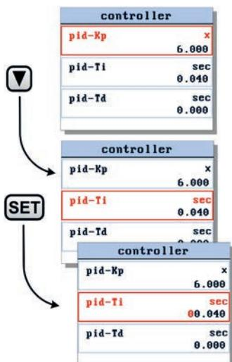
In the pid-controller settings screen you can select one of the PID parameters using the **▲** and **▼** buttons. Press **SET** to enter the edit mode.
