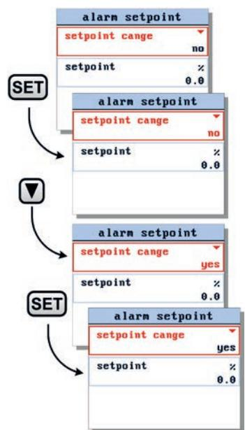
When entering the alarm setpoint settings screen the setpoint change parameter is selected. Press **SET** to enter the edit mode.
