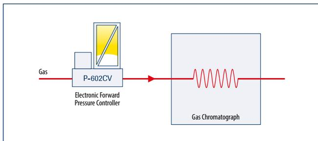
In Gas-Chromatography there is an increasing need to automate all required parameters. The EL-PRESS Forward Pressure Controller enables the user to select a desired pressure profile for the analyses, whereby the pressure is kept constant to a very precise value, even at very low flow rates.
