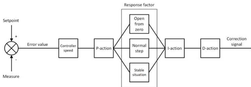
The controller speed controls the overall performance of the controller algorithm. Basically, to adjust the controller response, only the controller speed needs to be changed.
