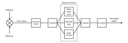
The <u>controller speed</u> controls the overall performance of the controller algorithm. Basically, to adjust the controller response, only the controller speed needs to be changed.
