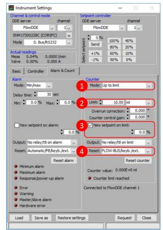
In the table below, the digital counter parameters are described from a batch dosing point of view. See <u>counter parameters</u> for usage and supported values.
