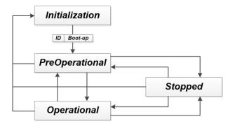
The CANopen NMT state machine effects the operation of the instrument. The Safe State functionality of the instrument is connected to the NMT state.
