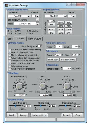
The response settings influence the controller gain by a factor depending on the stage the controller is in. The extra factor influences the controller gain as follows, in which a setting of 128 has no effect:
