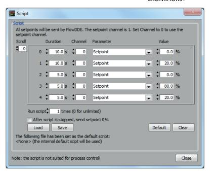
In the channel box, the value '0' can be set to let FlowPlot use the setpoint channel. The current setpoint channel is presented at the top of the window. The amount of repeats for this script can be adjusted, which can be set to infinite by entering '0'.
