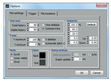
At Mode, the way the graph behaves when the plot reaches the 'end' of the time axis, can be selected:
